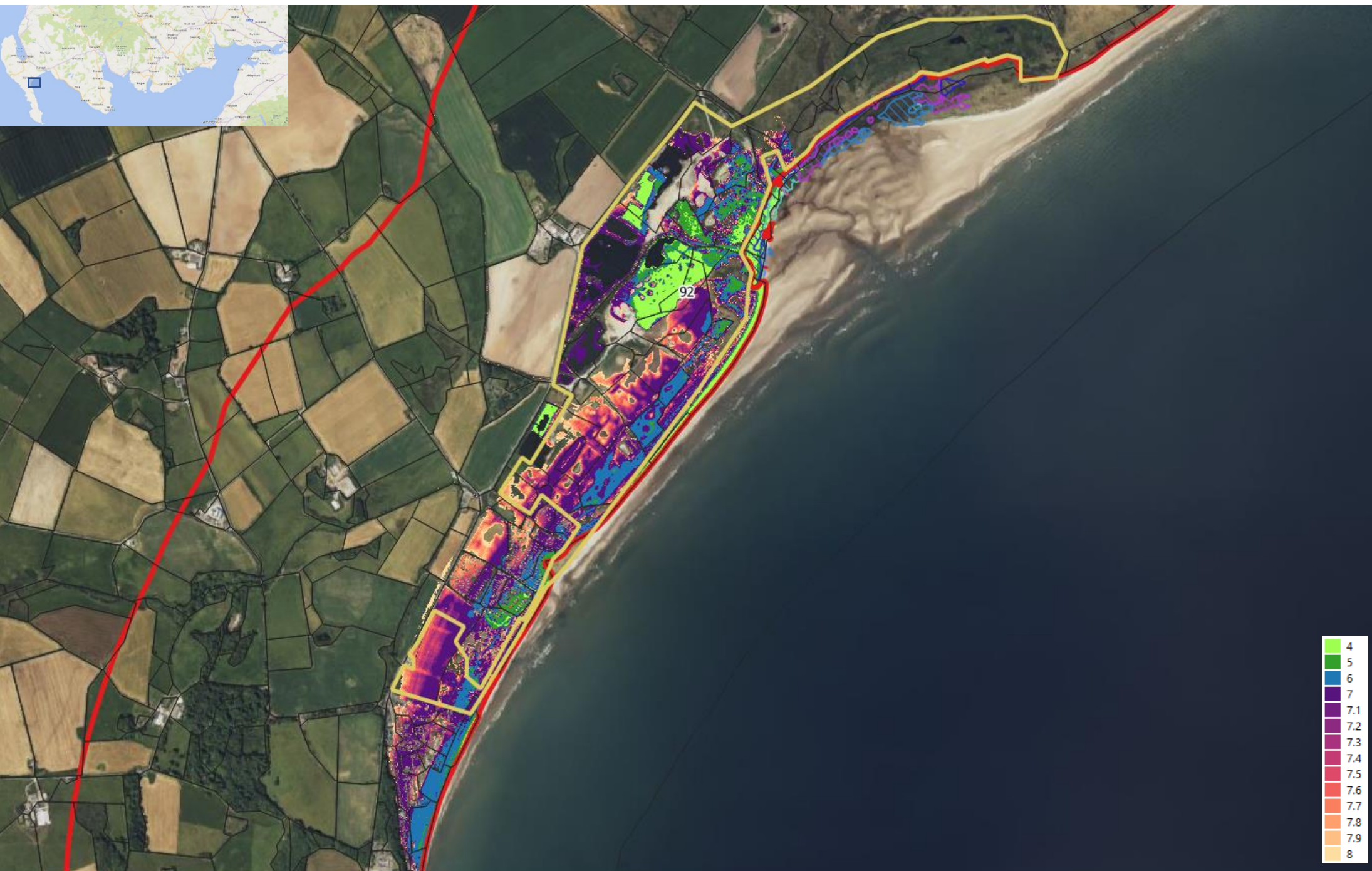
Saltmarsh opportunity mapping from east to west for D&G for site 92 spanning the north Solway for Clayshant, Luce Sands. Coloured site polygon boundaries shown alongside hatched areas of NVC "SM-prefix" habitat types. Red lines denote mean high water springs and its "buffer" to 1.5km inland. Field boundaries overlaid onto BING imagery .
